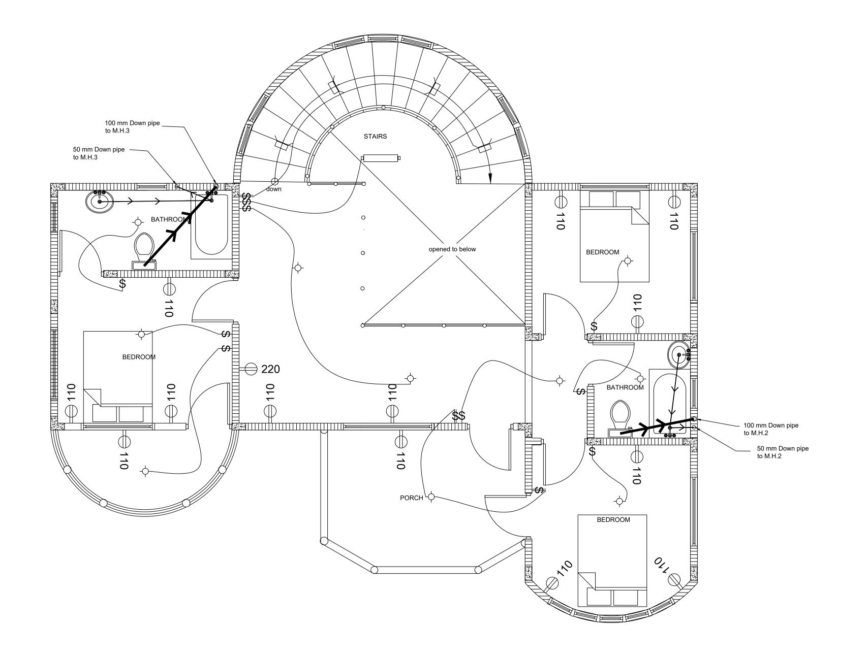
Electrical & Drainage Plan Scale: 1:40
